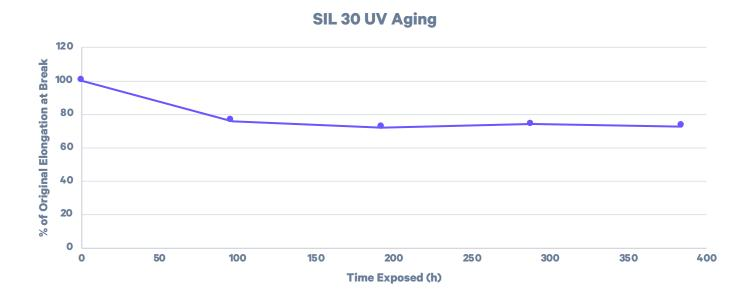
ASTM D4459: Q-Sun XE-1, 0.8 W/m² at 420 nm, 55  $^{\circ}\text{C}$  ASTM D412: Die C, 500 mm/min, average values represented
