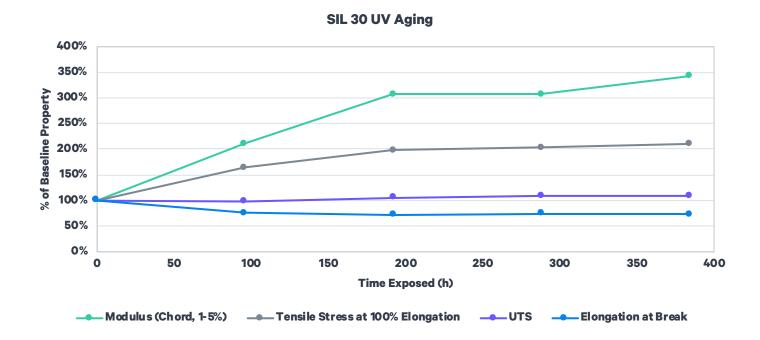
ASTM D4459: Q-Sun XE-1, 0.8 W/m² at 420 nm, 55  $^{\circ}\text{C}$  ASTM D412: Die C, 500 mm/min, average values represented
