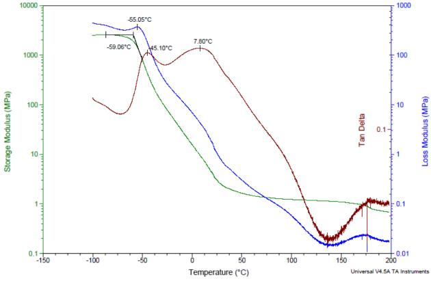
Standard: ASTM D4065 Instrument: TA DMA Q800 DMA Mode: Tension
