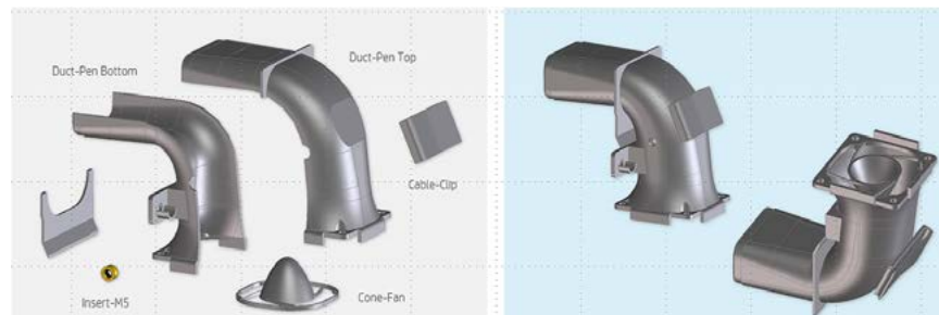
Figure 14: Maintain the integration of the functional design intent
